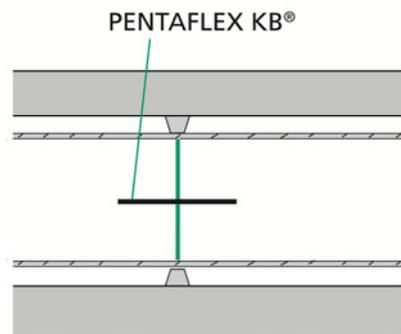
PENTAFLEX FTS – for controlled crack joints in pre-cast elements
