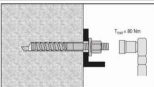
The required installation torque moment is given in Table B1.
