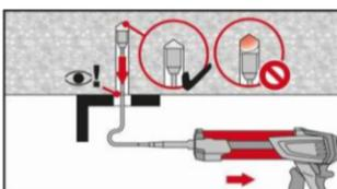
For overhead installation the injection is only possible with the aid of extensions and piston plugs. Assemble HIT-RE-M mixer, extension(s) and appropriately sized piston plug HIT-SZ 18. Insert piston plug to back of the hole and inject adhesive. During injection the piston plug will be naturally extruded out of the drill hole by the adhesive pressure.
