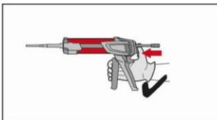
After injection is completed, depressurize the dispenser by pressing the release trigger. This will prevent further adhesive discharge from the mixer.
