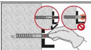
Mark the element and check the setting depth. The element has to fit in the hole until the required embedment depth. If it is not possible to insert the element to the required embedment depth, remove the dust in the drill hole or drill deeper.
