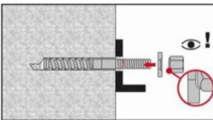
Orient round part of the nut to the conical washer and install.
