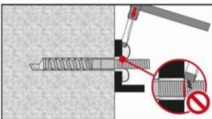
Do not damage thread of HIT-Z(-R)-D while removing excess mortar.
