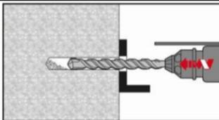
Through-setting: Drill hole through the clearance hole in the fixture to the required drilling depth with a hammer drill set in rotation-hammer mode using an appropriately sized carbide drill bit.
