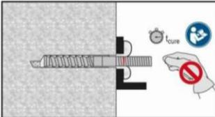
After required curing time  $t_{cure}$  (see Table B4) remove excess mortar.
