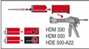
Tightly attach Hilti mixing nozzle HIT-RE-M to foil pack manifold. Do not modify the mixing nozzle.
