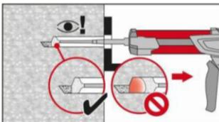
Inject the adhesive starting at the back of the hole, slowly withdrawing the mixer with each trigger pull.
