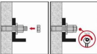
Apply the lock nut and tighten with a  $\frac{1}{4}$  to  $\frac{1}{2}$  turn. The anchor can be loaded.
