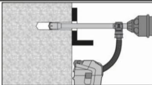
Through-setting: Drill hole to the required embedment depth with an appropriately sized Hilti TE-CD or TE-YD hollow drill bit with Hilti vacuum attachment. This drilling system removes the dust and cleans the drill hole during drilling when used in accordance with the user's manual (see Annex A1 - Borehole condition ②).
