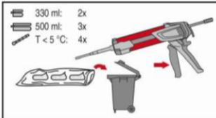
The foil pack opens automatically as dispensing is initiated. Depending on the size of the foil pack an initial amount of adhesive has to be discarded. Discarded quantities are:
