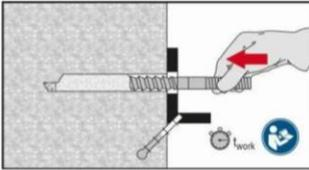
Before use, verify that the element is dry and free of oil and other contaminants. Set element to the required embedment depth before working time  $t_{work}$  has elapsed. The working time  $t_{work}$  is given in Table B4. After setting the element the annular gap between the anchor and the fixture (through-setting) has to be completely filled with mortar.
