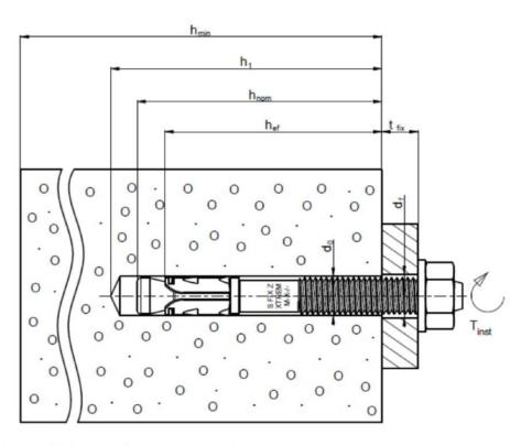
h<sub>min</sub>: Minimum thickness of concrete memberh<sub>1</sub>: Depth of drilled hole to deepest point
