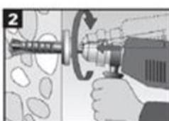
Once the FZUB depth stop meets the concrete, create the drill hole undercut by making circular swiveling movements with the hammer drill while the hammer mechanism is engaged. Press the hammer drill firmly against the anchor base: 1-2 swiveling movements are sufficient for  $\varnothing 14$  mm, with 3-5 movements for  $\varnothing 18$  mm and  $\varnothing 22$  mm
