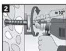
Once the FZUB depth stop meets the fixture, create the drill hole undercut by making circular swiveling movements with the hammer drill while the hammer mechanism is engaged. Press the hammer drill firmly against the anchor base: 1-2 swiveling movements are sufficient for  $\varnothing 14$  mm, with 3-5 movements for  $\varnothing 18$  mm and  $\varnothing 22$  mm
