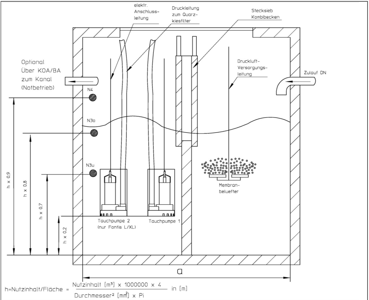
$$h = \frac{\text{Nutzinhalt [m}^3\text{]} \times 1000000 \times 4}{\text{Durchmesser}^2 \text{ [mm}^2\text{]} \times \text{Pi}} \text{ in [m]}$$
