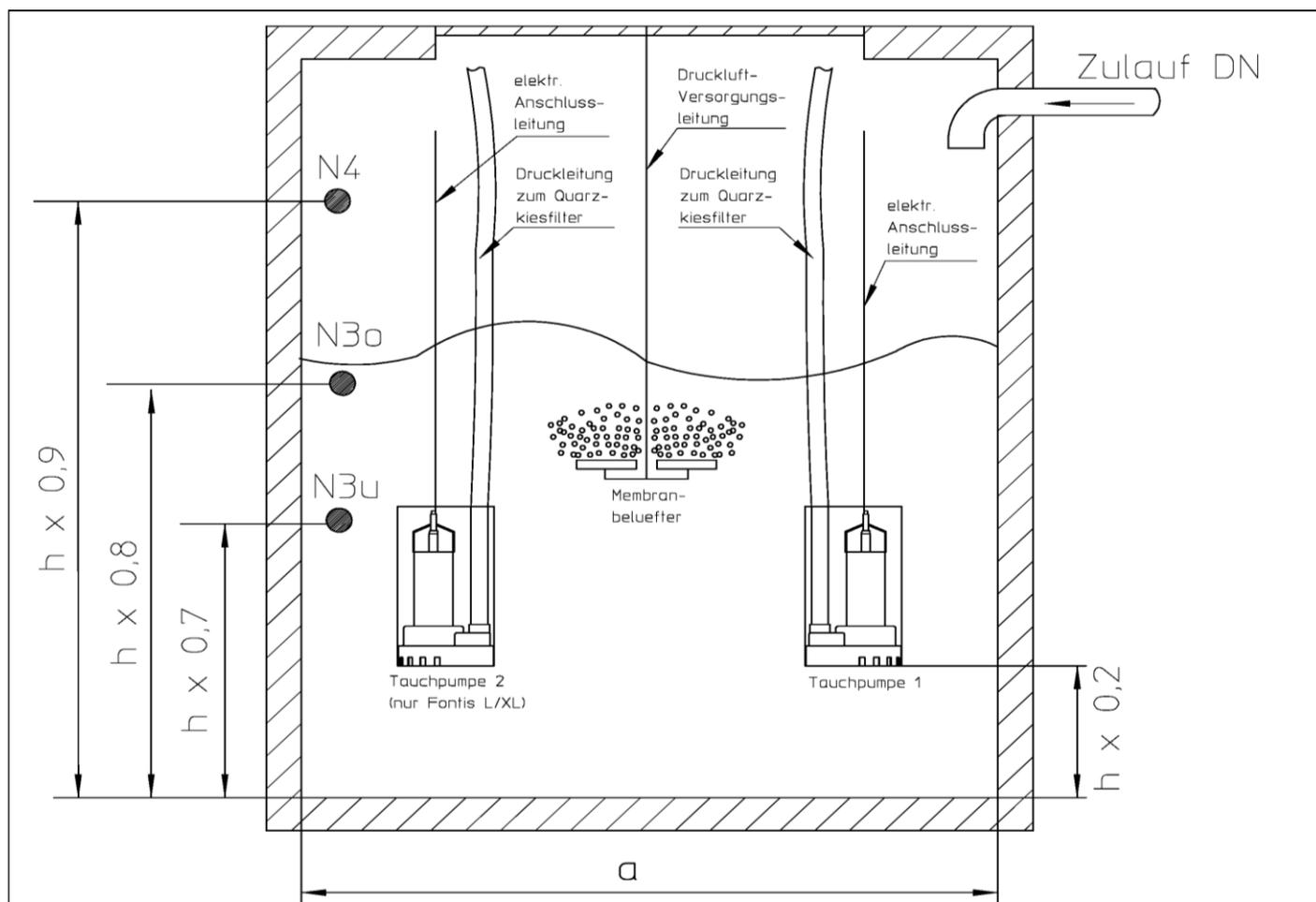
$$h = \frac{\text{Nutzinhalt [m}^3\text{]} \times 1000000 \times 4}{\text{Durchmesser}^2 \text{ [mm]} \times \pi} \text{ in [m]}$$
