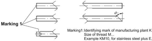
Size of thread M... Example KM10, for stainless steel plus E, for high corrosion plus H
