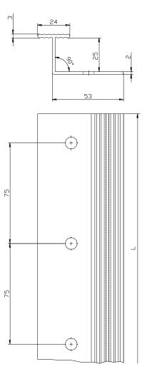
Vertical connection profile - "PVC Verbindungsleiste BM 400" (dimensions in millimetres)
