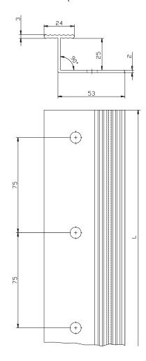
Vertical connection profile "Verbindungsleiste PVC" (dimensions in millimetres)
