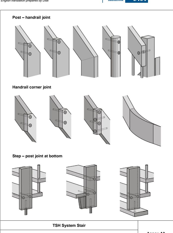
Post - handrail joint, handrail corner joint, Step – post joint
