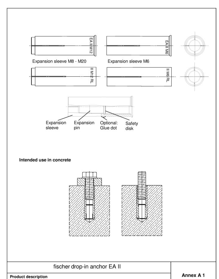
Anchor types Installed condition
