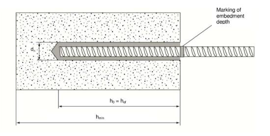
d<sub>f</sub> = diameter of clearance hole in the fixture
