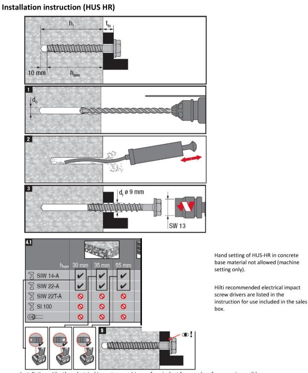
Installation with other electrical impact screw drivers of equivalent force and performance is possible.
