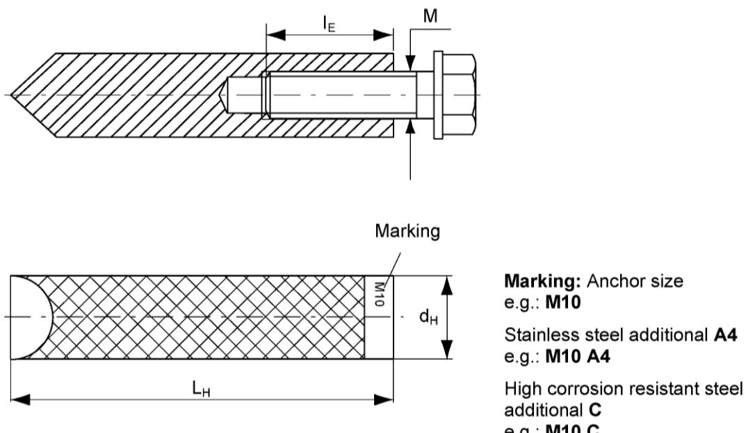
Retaining bolt or threaded rods (including nut and washer) must comply with the appropriate material and strength class of Annex A 3, Table A1
