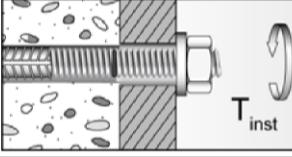
Mounting the fixture<br>$T_{\text{inst,max}}$ see Table B5                                                                            |
