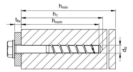
Nominal drill bit diameter  $d_0$ Nominal anchorage depth  $h_{nom}$ Depth of the drill hole  $h_1$
