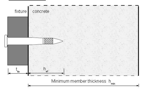
Powers Trak-It<sup>®</sup> XH and HD Nails for gas actuated tools C4 und C5
