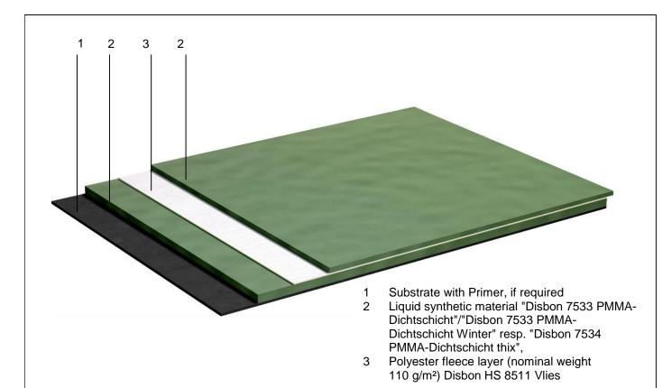
Applicable to the roof waterproofing "Disbon 7533 PMMA-Dichtschicht", "Disbon 7534 PMMA-Dichtschicht thix" and "Disbon 7533 PMMA-Dichtschicht Winter"
