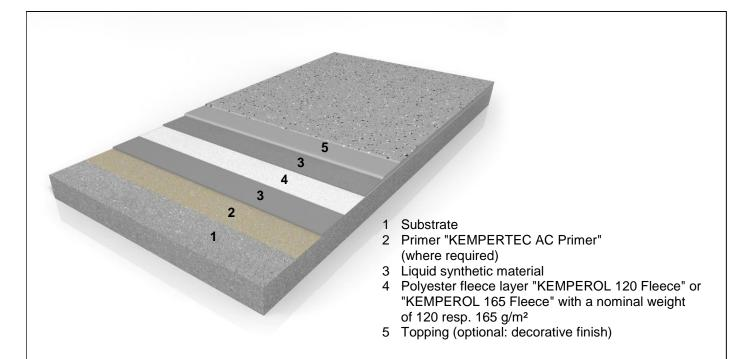
Applicable to the roof waterproofing "KEMPEROL AC Speed" / "KEMPEROL AC Speed+"
