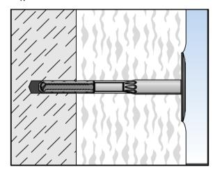
4. Correctly installed anchor
