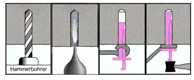
Hammer drilling only – keep installation parameters
