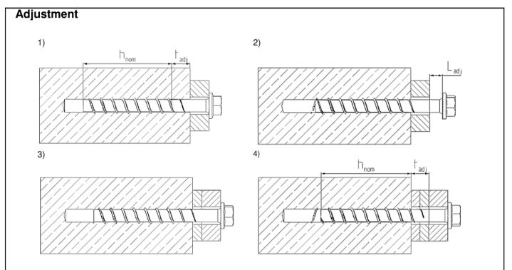
It is permissible to untighten the screw up to two times for adjustment purposes. Therefor the screw may be untighten to a maximum of  $L_{adj} = 20$  mm off the surface of the initial fixture. The total permissible thickness of shims added during the adjustment process is  $t_{adj} = 10$  mm.
