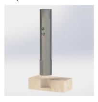
2. Check the correct hole dimension with the GO / NO GO measuring gauge
