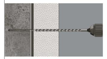
Drill the hole perpendicular to the substrate surface. Clean the drill hole 3x.
