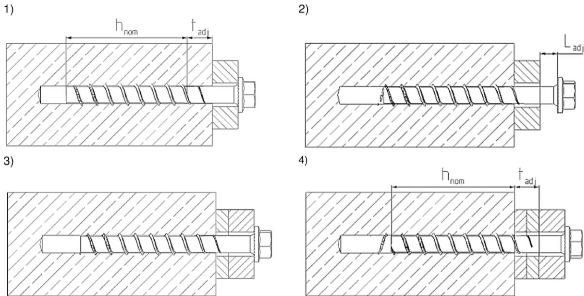
It is permissible to untighten the screw up to two times for adjustment purposes.
