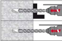
**Through-setting:** Drill hole through the clearance hole in the fixture to the required drilling depth with a hammer drill set in rotation-hammer mode using an appropriately sized carbide drill bit.
