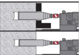
Diamond coring is permissible when a suitable diamond core drilling machine and corresponding core bit are used.
