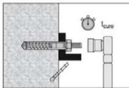
After required curing time  $t_{cure}$  (see Table B4 or Table B5) remove excess mortar. The required installation torque  $T_{inst}$  is given in Table B1. The anchor can be loaded.
