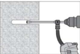
**Pre- / Through-setting:** Drill hole to the required embedment depth with an appropriately sized Hilti TE-CD or TE-YD hollow drill bit with Hilti vacuum attachment. This drilling system removes the dust and cleans the drill hole during drilling when used in accordance with the user's manual (see Annex A1 - Borehole condition ©).
