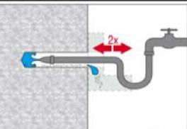
Flush 2 times from the back of the hole over the whole length until water runs clear. Water-line pressure is sufficient.
