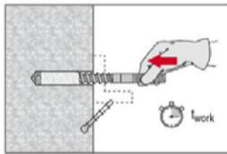
Before use, verify that the element is dry and free of oil and other contaminants. Set element to the required embedment depth before working time  $t_{work}$  (see Table B4 or Table B5) has elapsed. After setting the element the annular gap between the anchor and the fixture (through-setting) or concrete (pre-setting) has to be filled with mortar.
