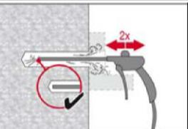
Blow 2 times from the back of the hole (if needed with nozzle extension) with oil-free compressed air (min. 6 bar at 6 m<sup>3</sup>/h) to evacuate the water.
