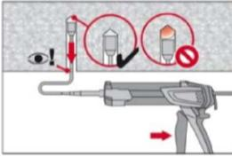
For overhead installation the injection is only possible with the aid of extensions and piston plugs. Assemble HIT-RE-M mixer, extension(s) and appropriately sized piston plug (see Table B6). Insert piston plug to back of the hole and inject adhesive. During injection the piston plug will be naturally extruded out of the drill hole by the adhesive pressure.
