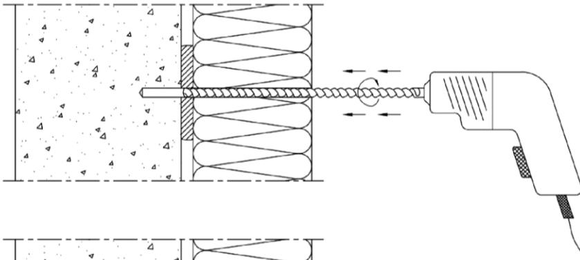
Drill the hole perpendicular to the substrate surface.
