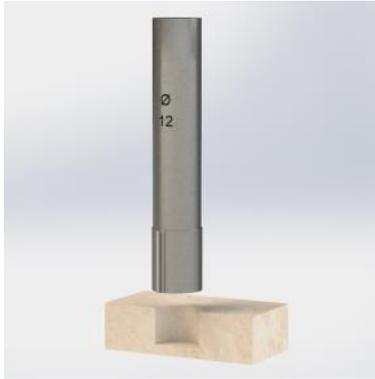
2. Check the correct hole dimension with the GO / NO GO measuring gauge
