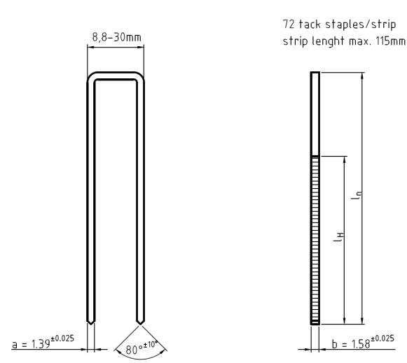
raw material: wire ø1,52± 0,01 made of steel 1.4301 (X 5 Cr Ni 18 10 = V2a) according DIN EN 10088-1 with a minimum tensile strength of 950  $\mathrm{N/mm}^2$
