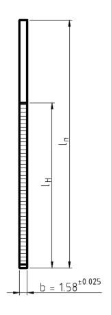
raw material: wire  $\emptyset$ 1,52±0,01 made of steel according DIN EN ISO 16120 with a minimum tensile strength of 900 N/mm<sup>2</sup> glue: type 3 according DIN EN 14592:2008+A1:2012, according to the manufacturer declaration surface: strong galvanized with a layer thickness of at least 12 $\mu$
