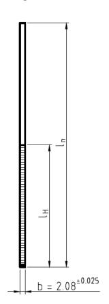
raw material: wire  $\phi$ 2,00±0,01 made of steel according DIN EN ISO 16120 with a minimum tensile strength of 900 N/mm<sup>2</sup> glue: type 3 according DIN EN 14592:2008+A1:2012, according to the manufacturer declaration surface: strong galvanized with a layer thickness of at least 12 $\mu$
