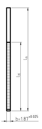
raw material: wire  $\phi$ 1,80±0,01 made of steel according DIN EN ISO 16120 with a minimum tensile strength of 900 N/mm<sup>2</sup> glue: type 3 according DIN EN 14592:2008+A1:2012, according to the manufacturer declaration surface: strong galvanized with a layer thickness of at least 12 $\mu$
