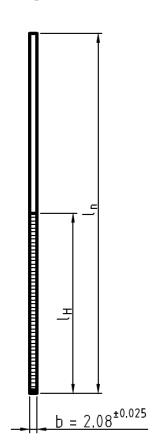
raw material: wire  $\emptyset$ 2,00 ±0,01 made of steel 1.4301 (X 5 Cr Ni 18 9 = V2a) according DIN EN 10088–1 with a minimum tensile strength 950 N/mm<sup>2</sup>
