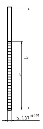
raw material: wire  $\phi$ 1.80±0.01 made of steel 1.4301 (X 5 Cr Ni 18 9 = V2a) according DIN 10088-1 with a minimum tensile strength of 950 N/mm<sup>2</sup>
