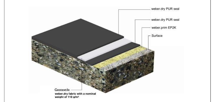
Applicable to the roof waterproofing "weber.dry PUR seal"
