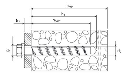
$\begin{array}{lll} d_0 & = & \text{nominal drill hole diameter} \\ h_{\text{nom}} & = & \text{nominal embedment depth} \\ h_1 & = & \text{depth of the drill hole} \\ h_{\text{min}} & = & \text{minimum thickness of member} \\ t_{\text{fix}} & = & \text{thickness of fixture} \end{array}$
