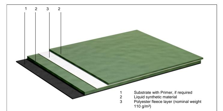
Applicable to the roof waterproofing "Renolit Poliquid Infinite", "Renolit Poliquid Detail" and "Renolit Poliquid Infinite MX":
