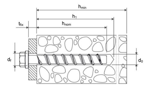
$\begin{array}{lll} d_0 & = & \text{nominal drill bit diameter} \\ h_{\text{nom}} & = & \text{nominal anchorage depth} \\ h_1 & = & \text{depth of the drill hole} \\ h_{\text{min}} & = & \text{minimum thickness of member} \end{array}$
