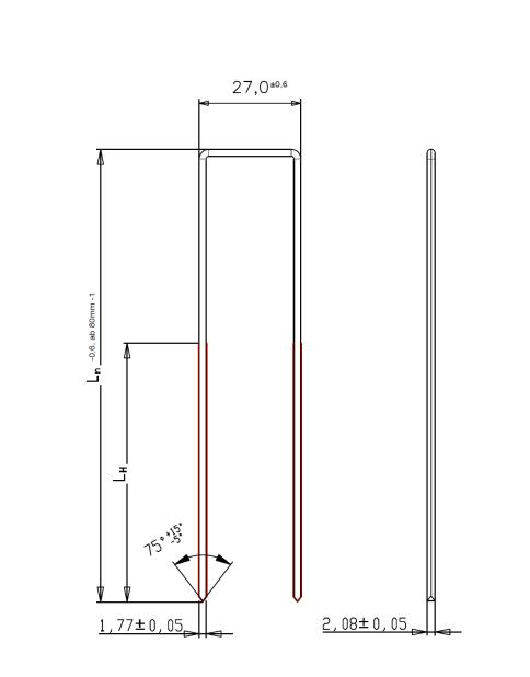
Staple raw wire: Round stainless steel  $\emptyset$  2,00±0,03mm Tensile strength  $\ge$  900 N/mm<sup>2</sup> WNr. 1.4301 / 1.4401 or 1.4529 Leg length L<sub>n</sub> = 35,0 - 170,0mm
