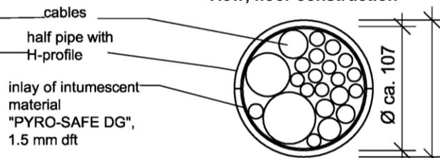
"PYRO-SAFE CT Cable Tube" and "PYRO-SAFE CT ML Cable Tube"
