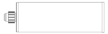
235 ml, 345 ml and 825 ml cartridge (Type: "side-by-side")
