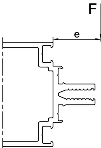
$$e = \max.t_{\text{Glas}} / 2 + t_{\text{Gummileiste}} = 45 \text{ mm}$$
