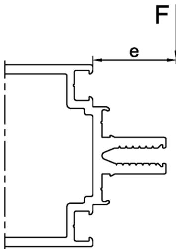
$$e = \max.t_{\text{Glas}} / 2 + t_{\text{Gummileiste}} = 45 \text{ mm}$$
