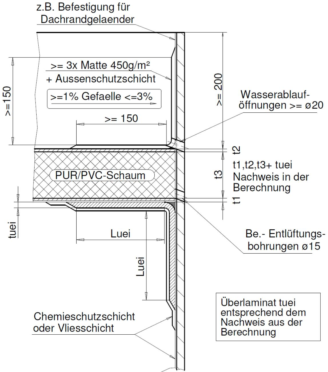
$t_{uei} \geq 3 \times \text{Matte } 450\text{g/m}^2$
