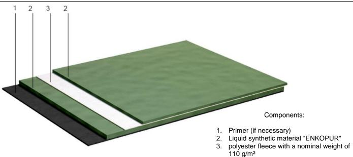
Applicable to the roof waterproofing "ENKOPUR"
