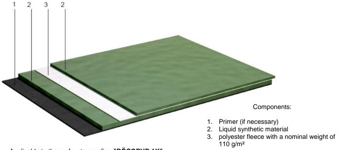
Applicable to the roof waterproofing "BÖCOPUR 1K"
