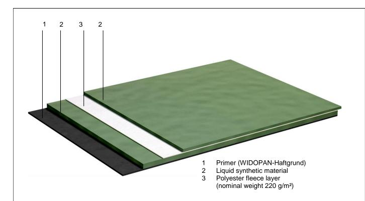
Applicable to the roof waterproofing "WIDOPAN-FD" / "WIDOPAN-Plus":
