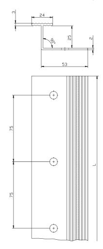
Vertical connection profile "Brillux WDVS Verbindungsleiste 3544" (dimensions in millimetres)
