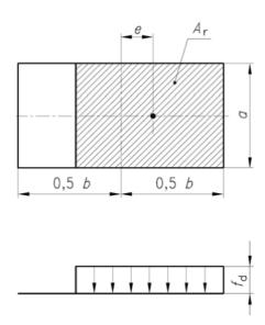
Figure I.2 - Reduced contact area A<sub>r</sub> for rectangular sliding surfaces.
