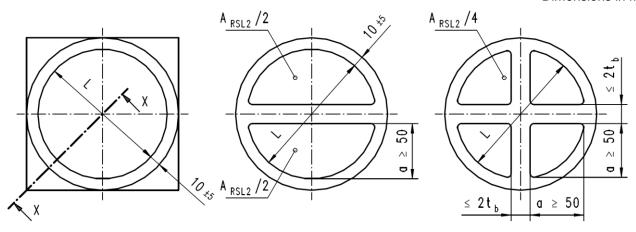
Figure H.2 - Examples of recessed flat ROBO®SLIDE L2 configurations
