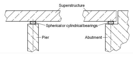
Figure A.1 - Assembly of a guided and free movable mageba RESTON®Spherical and Cylindrical Bearings and its intended use (example)
