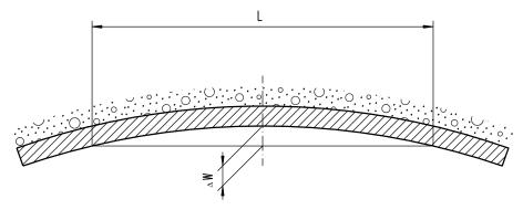
Figure F.1 - Deformations of backing plates.
