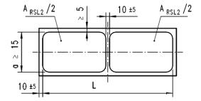
Figure H.4 - Examples of recessed ROBO®SLIDE L2 sheets for guides
