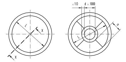
Figure H.3 - Subdivision of recessed ROBO®SLIDE L2 sheets for spherical sliding surfaces
