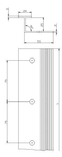
Vertical connection profile "DHTherm Verbindungsschiene" (dimensions in millimetres)
