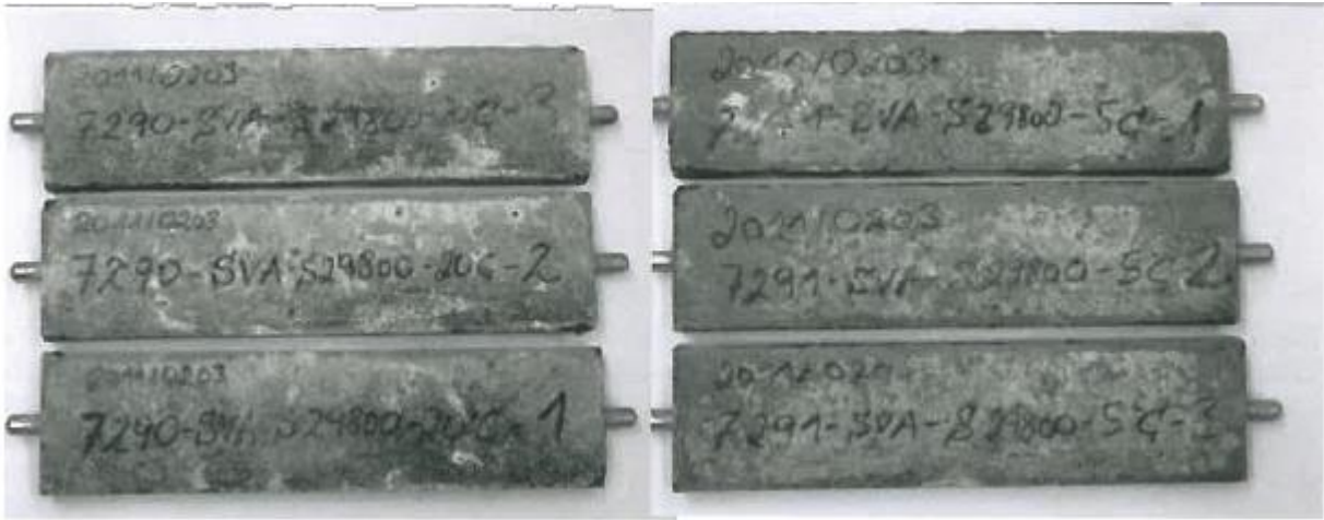
Figure A3: Specimens with CEM I 42,5 R-SR0 after 180 days; Na 2 O 4 -Lösung Solution: 20 °C-storage (on the left) and 5 °C-storage (on the right)
