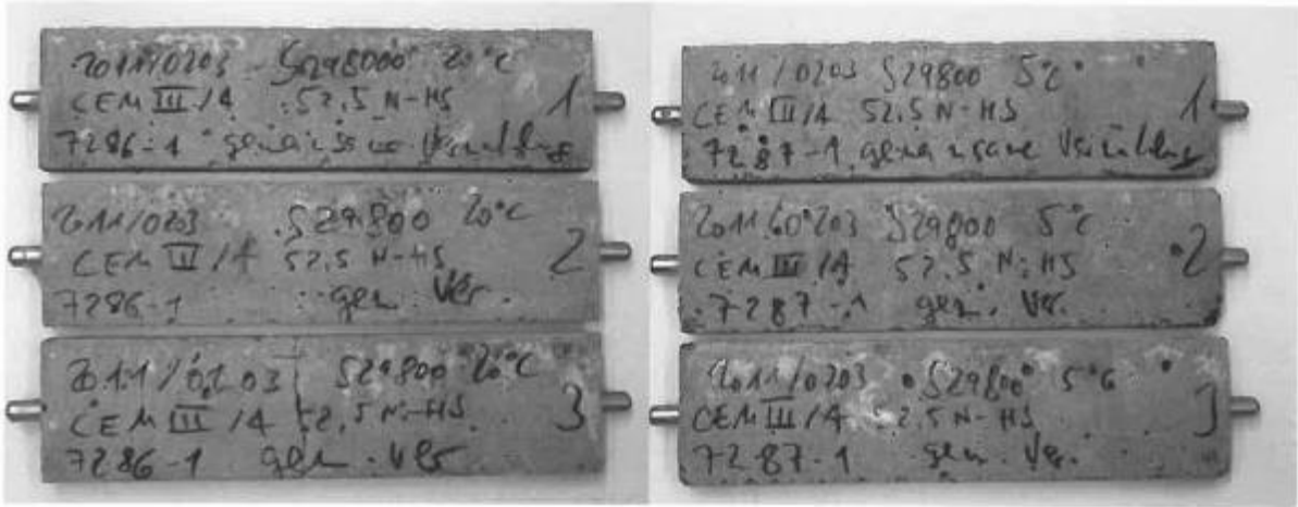
Figure A1: Specimens with CEM III/A 52,5 N-SR "Ennigerloh" after 180 days; Na_2O_4 -Lösung Solution: 20 °C-storage (on the left) and 5 °C-storage (on the right)
