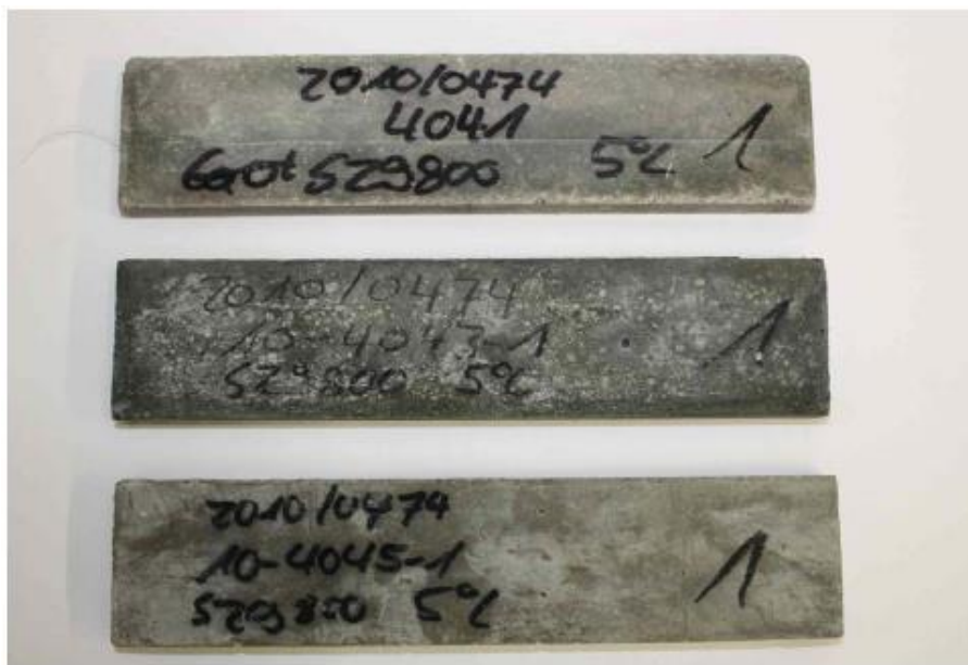
Figure A2: Flat prism after 180 days storage in Na 2 SO 4 -solution at 5 °C (top: prism from CEM III/A 42,5 N-LH/SR/LA "Deuna" (C1) with blast furnace slag 1 (S1); mid: CEM I 42,5 N-SR0; bottom: CEM III/B 42,5 N-LH/SR)
