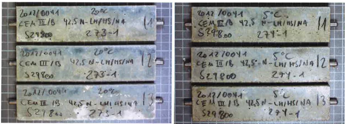
Figures A4: Flat prism from blast furnace cement CEM III/B 42,5 N-LH/SR after 180 days storage in Na 2 SO 4 -solutions at 20 °C (on the left) and 5 °C (on the right)
