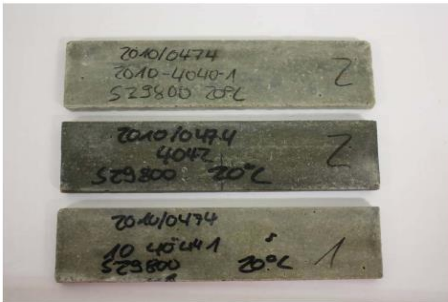
Figure A1: Flat prism after 180 days storage in Na 2 SO 4 -solution at 20 °C (top: prism from CEM III/A 42,5 N-LH/SR/LA "Deuna" (C1) with blast furnace slag 1 (S1); mid: CEM I 42,5 N-SR0; bottom: CEM III/B 42,5 N-LH/SR)
