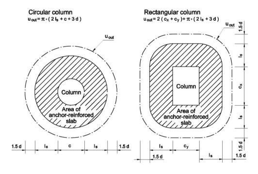
HALFEN HDB double headed studs for punching shear reinforcement
