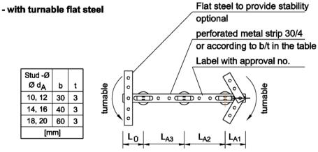
Material: A4 = 1.4571/ 1.4401/ 1.4404 (acc. to EN 10088-5:2009) S 235 JR = 1.0038 (acc.to EN10025-2:2004) DD11 = 1.0332 (acc. to EN10111:2008)
