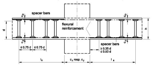
Concrete cover c₀ resp. cu acc. to EN1992-1-1: 2004 + AC: 2010, section 4.4
