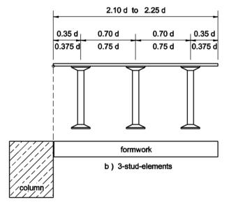
HALFEN HDB double headed studs for punching shear reinforcements
