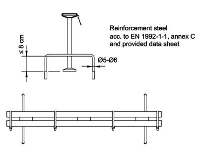
HALFEN HDB double headed studs for punching shear reinforcements
