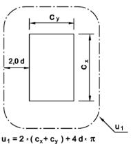
b) Loaded areas (columns) are less than 6d from openings (voids) in the slab.
