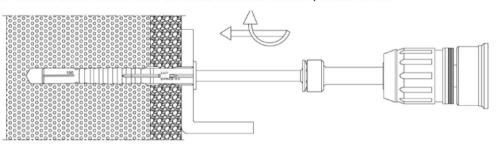
4. Correctly installed anchor
