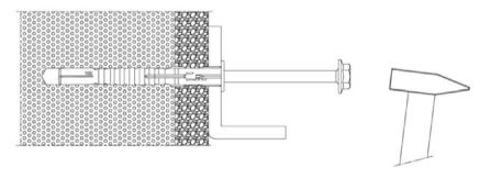
3. Screw in the screw until the head is rested on the plastic sleeve
