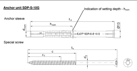
Picture 3: Dowel type countersunk (S)
