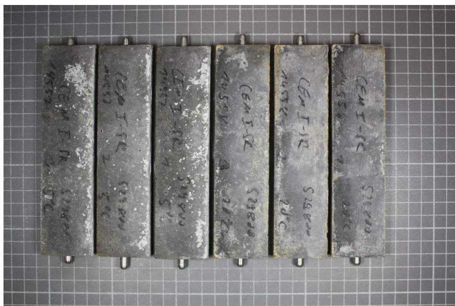
Figure A4: Specimens with CEM I 42,5 R-SR3 after 180 days; Storage: in \text{Na}_2\text{O}_4 -Solution at 5 °C (3 left-hand side specimens) and at 20 °C (3 right-hand side specimens)
