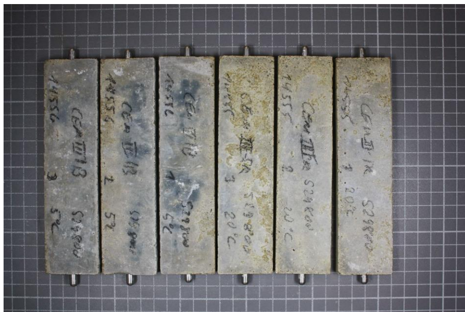
Figure A3: Specimens with CEM III/B 42,5 N-LH/SR after 180 days; Storage: in \text{Na}_2\text{O}_4 -Solution at 5 °C (3 left-hand side specimens) and at 20 °C (3 right-hand side specimens)
