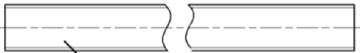
Hilti meter rod AM 8.8 electroplated zinc coated, AM HDG 8.8 hot dip galvanized M8 to M30, 1m to 3m
