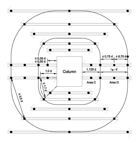
HALFEN HDB double headed studs for punching shear reinforcements Annex B7 Intended use HDB parallel arrangement in slabs
