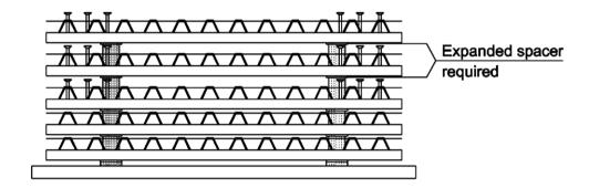
HALFEN HDB double headed studs for punching shear reinforcements
