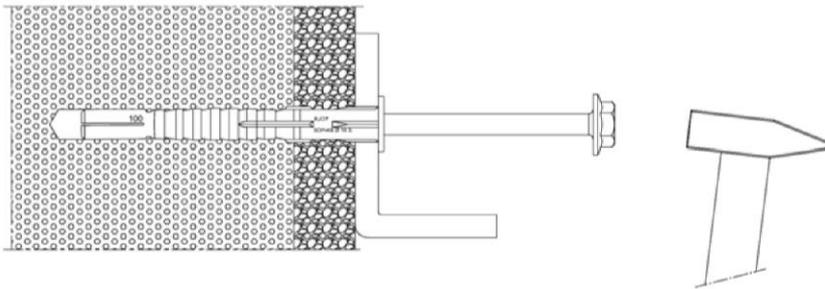
3. Screw in the screw until the head is rested on the plastic sleeve
