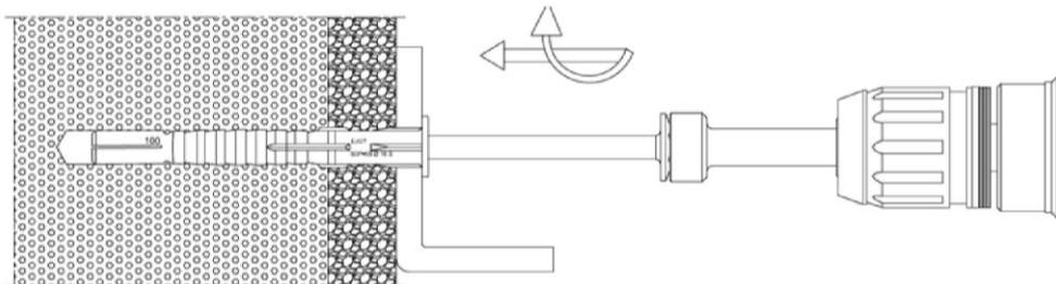
4. Correctly installed anchor
